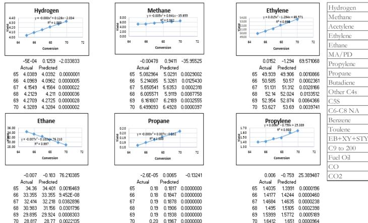
Similar regressed equations for Propane, Butane, Naphtha feed can be estimated for other component as show in above table. By using regressed equations and recovery model, the individual component flows in furnace effluent and for all in-out streams across columns/sections can be estimated.
